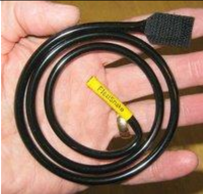
This tool is a smaller version of the plumber snake. It has Velcro on the end so that it will pick up hair that is clogging a drain.
